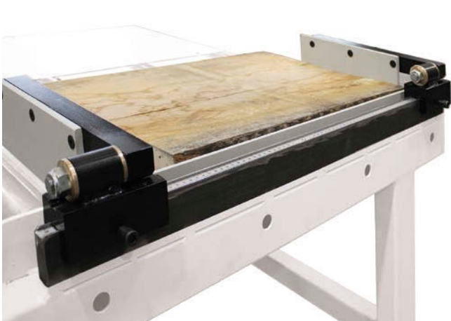
➤ Battuta meccanica Mechanic positive stop ✓cs700 ✓cs1000
