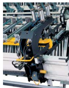
Hydraulic type with top press cylinders (KCCMO/H)
